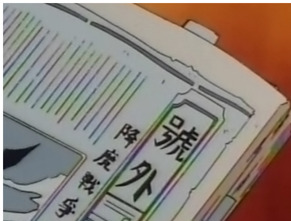
Figure 60: After two passes with Smart Smoother IQ, our scene has considerably less rainbowing than before.
