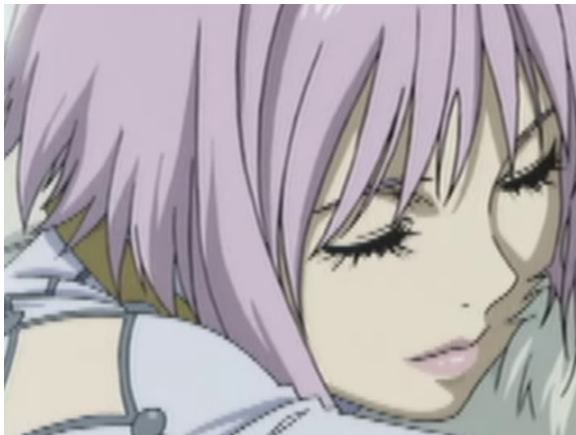
Figure 67: We slowed down our deinterlaced footage in Premiere, but by default, it tries to deinterlace the clip again using a very poor method of doing so. Not only are the edges jagged, but they wiggle as the video plays. It is very noticeable on both computer monitors and televisions.
