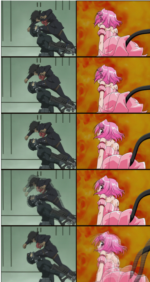
Figure 24: Examples of video encoded through different telecine procedures. On the left, Blue from Wolf's Rain shows off her legs, as well as properly telecined video through 3:2 pulldown. You can't see it well in the scaled-down image, but the last frame is slightly interlaced as well. On the right, Mew Ichigo shows us not only poor telecine (1 frame in 5 is interlaced) but if you look closely, the background is properly telecined, just not in sync with the rest of the animation! Background and character animators usually work separately, and these are the things that can result from a group effort gone bad. Fortunately, the background isn't moving much, so if we can just properly deinterlace Ichigo, our footage should be OK.
